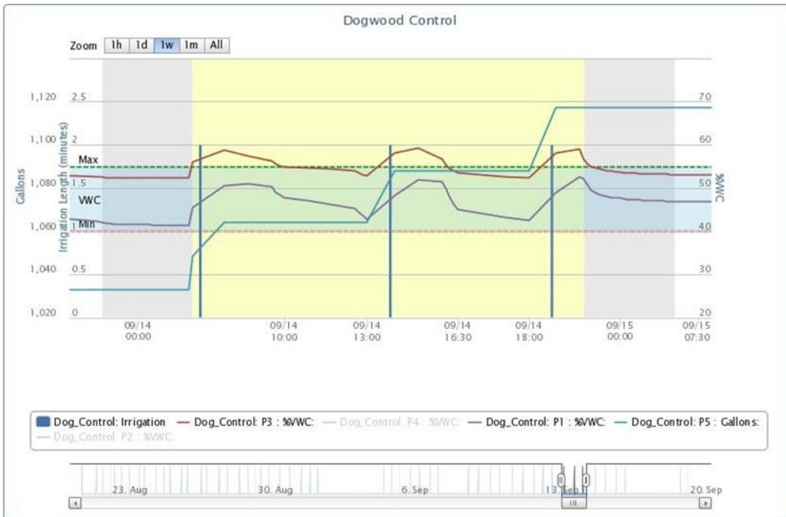
Fig. 9. Graphical display of data showing blue vertical bars (irrigation events) and horizontal data lines for two soil moisture sensors. The set-point average for control was maintained at 46% substrate volumetric water content during 2012. The light blue horizontal line shows real-time water use from the flow meters integrated into the system. The horizontal blue band is a user defined region that quickly indicates optimal moisture levels to the grower.
