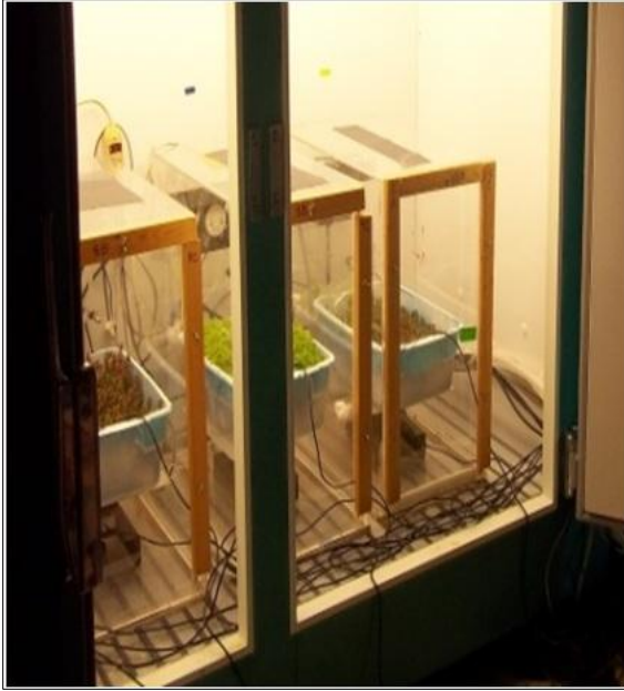
Fig. 65. Sedum in UGA growth chambers, enabling continuous gas exchange measurements of plants in each chamber.
