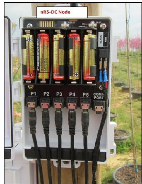
Fig.1. The nR5-DC sensor node installed in a pot-in-pot nursery in Tennessee
