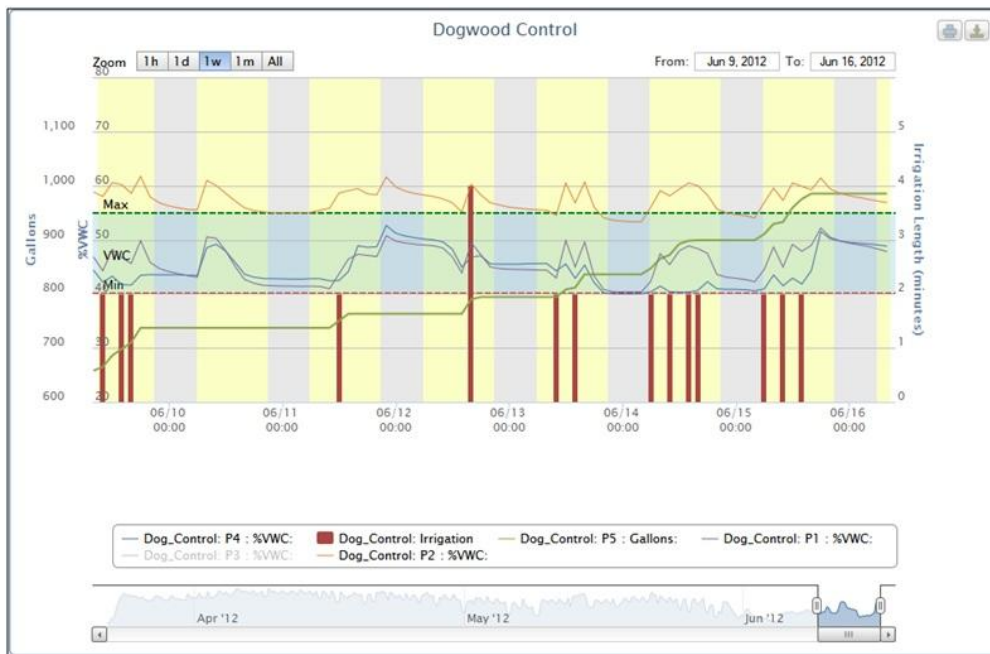
Fig. 59. A graph of substrate VWC from the10HS sensors in four individual trees (left axis) plotted by the Sensorweb software during June, 2012 for the controlled block. The red line indicates cumulative water applied per row of 133 trees (gallons; right axis)
