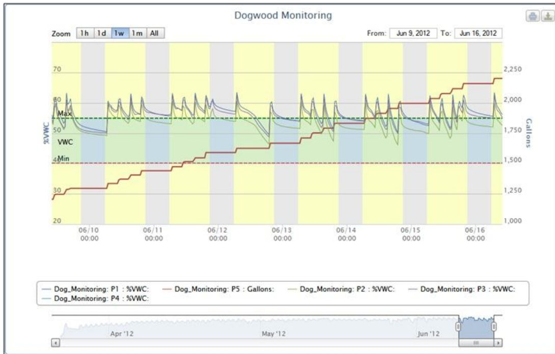
Fig. 58. A graph of substrate VWC from the10HS sensors in four individual trees (left axis) plotted by the Sensorweb software during June, 2012 for the monitored block. The red line indicates cumulative water applied per row of 133 trees (gallons; right axis)
